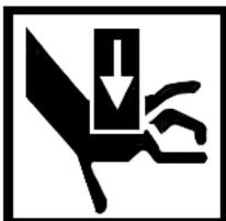
This warning symbol indicates the presence of possible dangerous pinch – points. Moving mechanical parts can crush and / or sever body parts.
