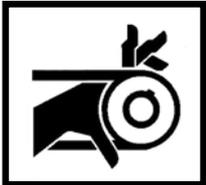
This warning symbol alerts you to the presence of possible dangerous drive mechanisms within the machine. Guards **should always be** in place when the machine is in operation.
