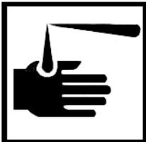
This warning symbol indicated the presence of possibly dangerous chemicals. Proper precautions **should be** taken when handling corrosive or caustic material.
